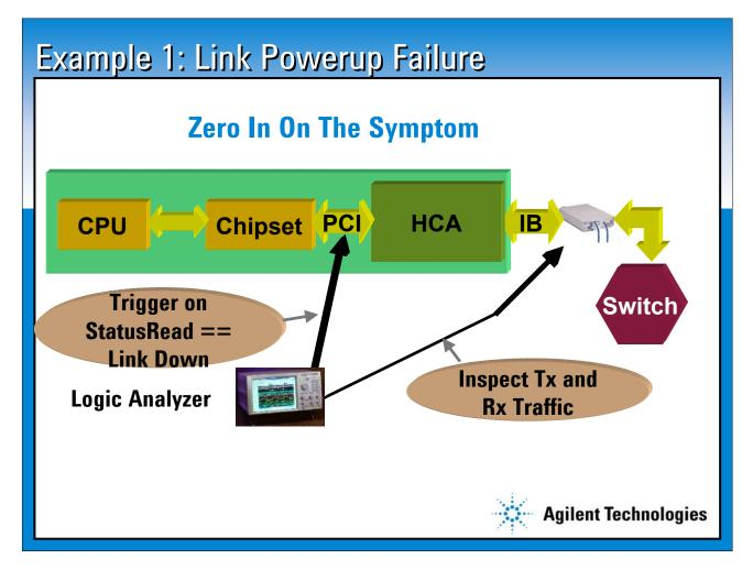
Example 1: Link Powerup Negotiation Failure Zero in on the Symptom
