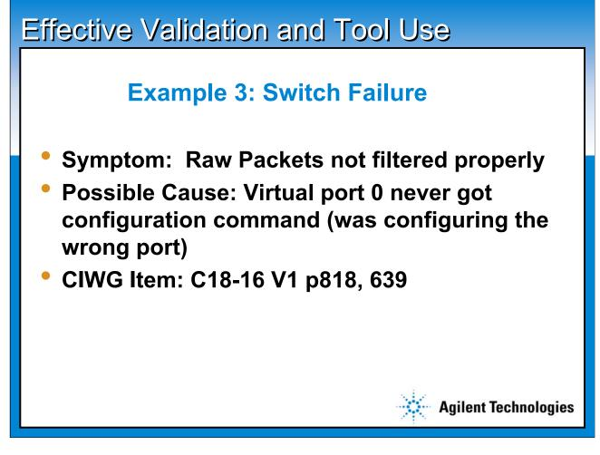
Switch Failure Example
