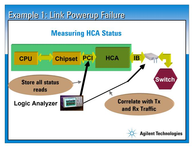
Example 1: Link Powerup Negotiation Failure Measuring HCA Status
