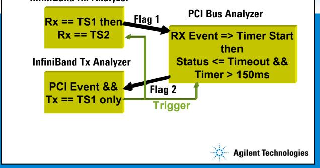
Example 1: Link Powerup Negotiation Failure Triggering on the Error
