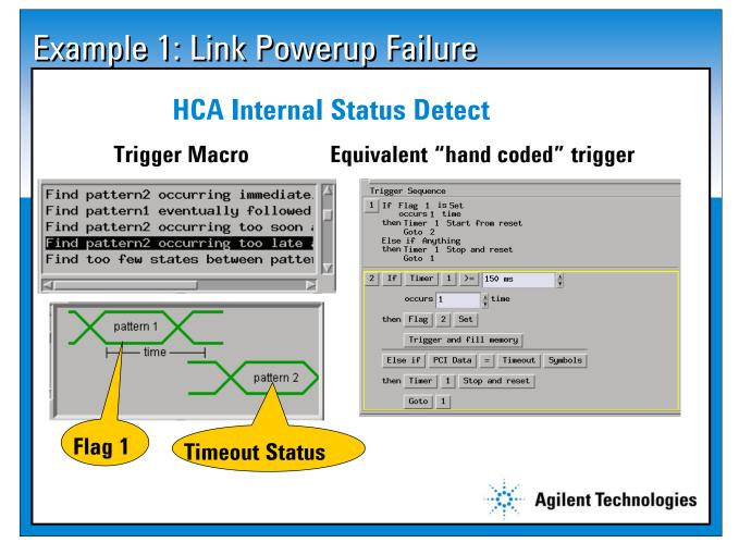
Example 1: Link Powerup Negotiation Failure HCA Internal Status Detect
